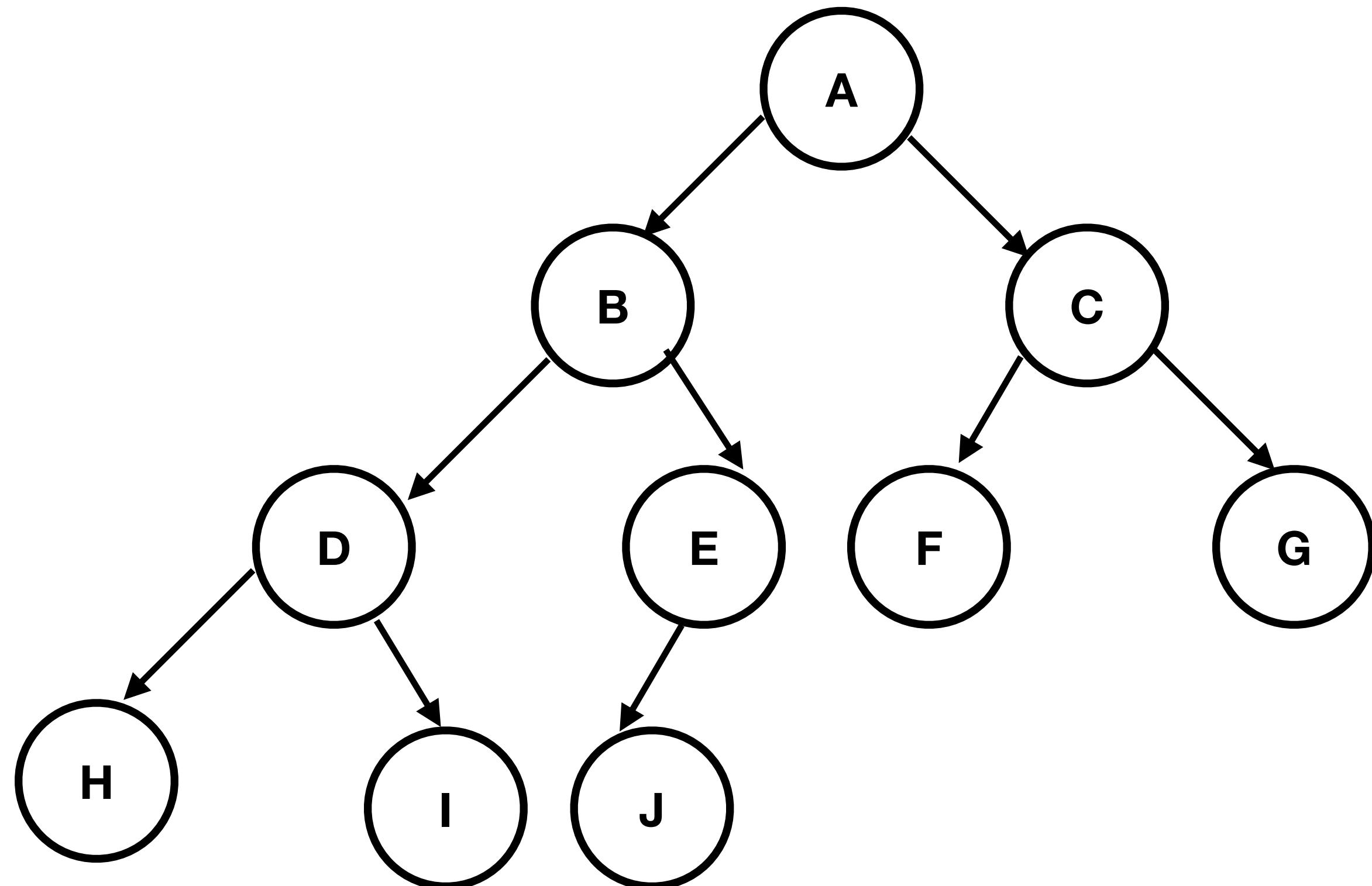
A **complete binary tree** is a binary tree in which every level but the deepest is full and the deepest level is either full or the nodes are as far left as possible.
