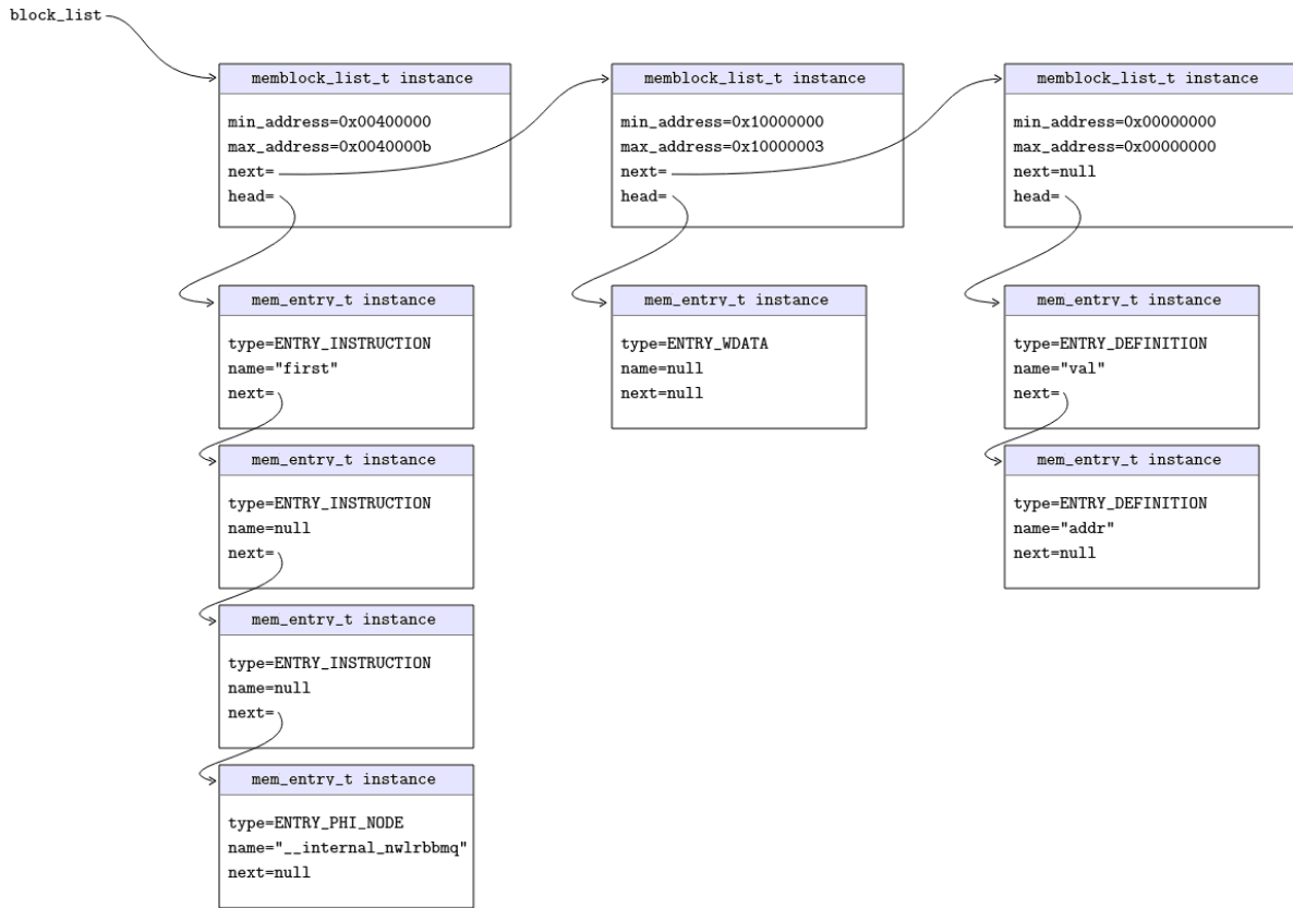
Figure 2. Internal data structure representation of an example .dt program.
